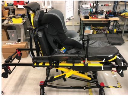
Figure 32 – Attach to the foot end extension tube
