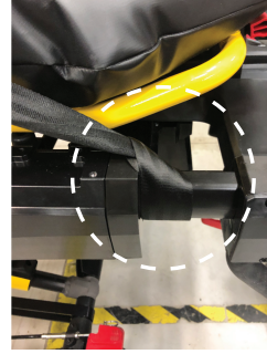
Figure 32 – Attach to the foot end extension tube
